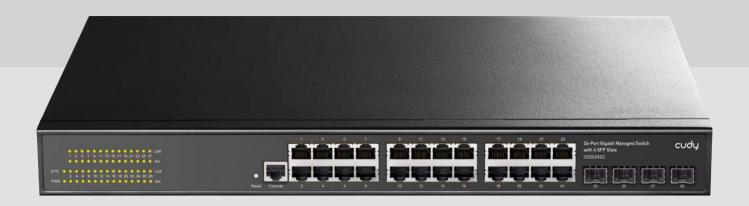
24-Port Gigabit Managed Switch with 4 SFP Slots
