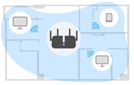
Beamforming, and four antennas combine to deliver focused reception to devices far away.
